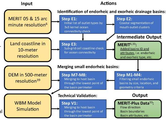
Flowchart of the workflow to produce the MERIT-Plus datasets. Left column objects are the processing inputs (tan); middle and right column objects are the processing actions (dark blue) and outputs (green).
